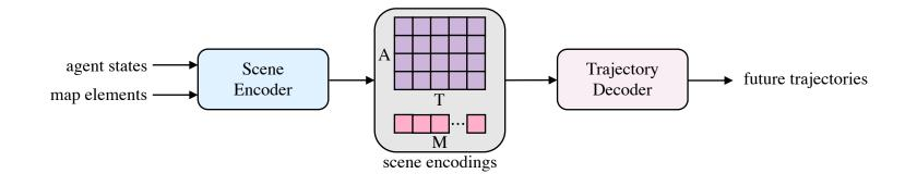
Agent encodings of shape [A, T, D] – A agents x T historical time steps x D hidden Scene encodings dimensions Map encodings of shape [M, D] – M map elements x D hidden dimensions
