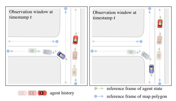
1. Set up a local spacetime coordinate system for each agent state and each map element that a query vector will derive from
