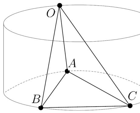
The danger cylinder is defined as a circular cylinder circumscribing points A,B,C with axis normal to the plane ABC
