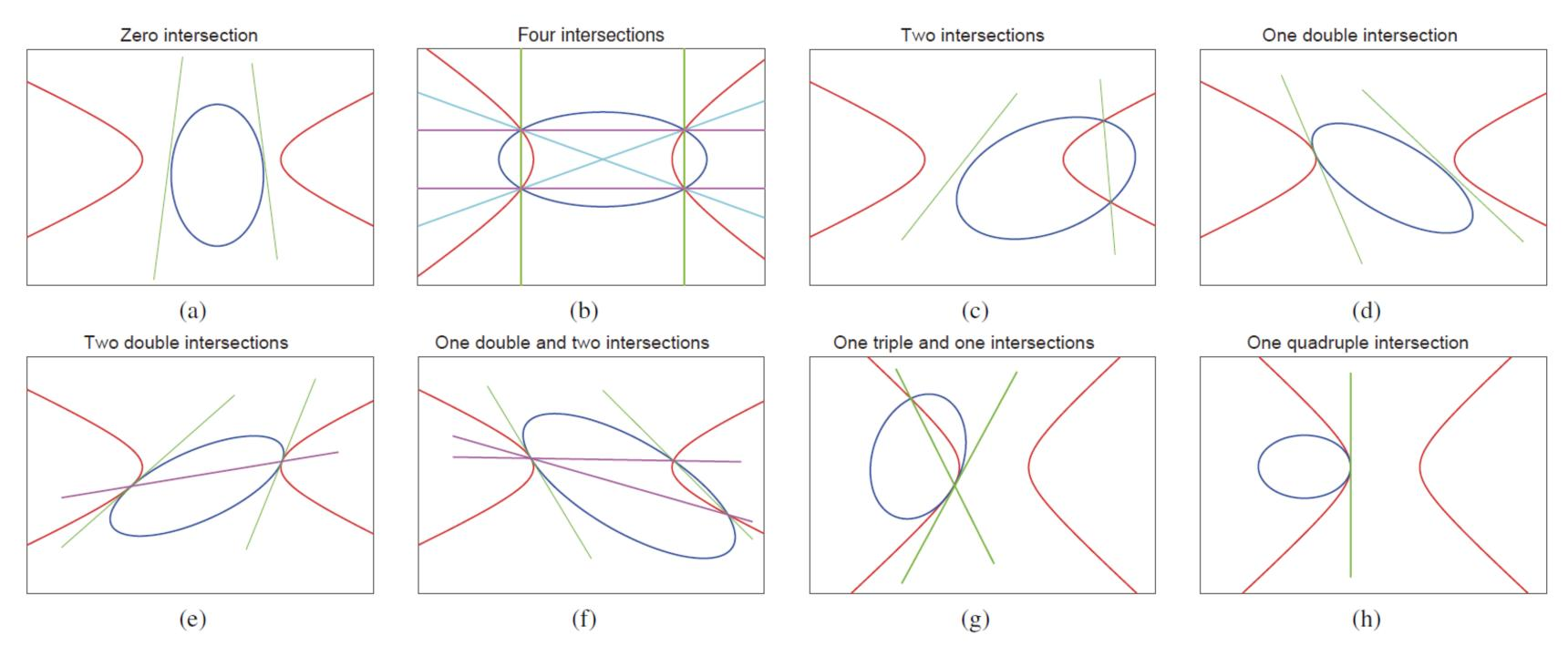
Illustration of eight possible cases for the relative position of a hyperbola and an ellipse. The pair of lines with different colors corresponds to different cubic roots.
