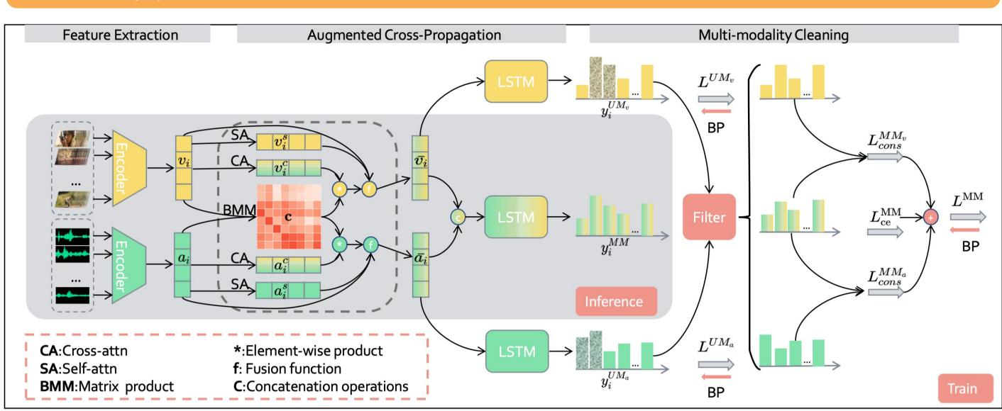
CLC includes three modules. The visual and audio modalities of the input video are represented as vectors by the feature extraction module. Then the features are augmented by ACP module to capture semantic associations across modalities. MMC is used to filter outs noisy and incomplete labeling with additional uni-modal branches.
