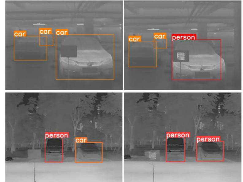
Figure 9. Examples of OAA and RAA for car misclassification in the physical world.
