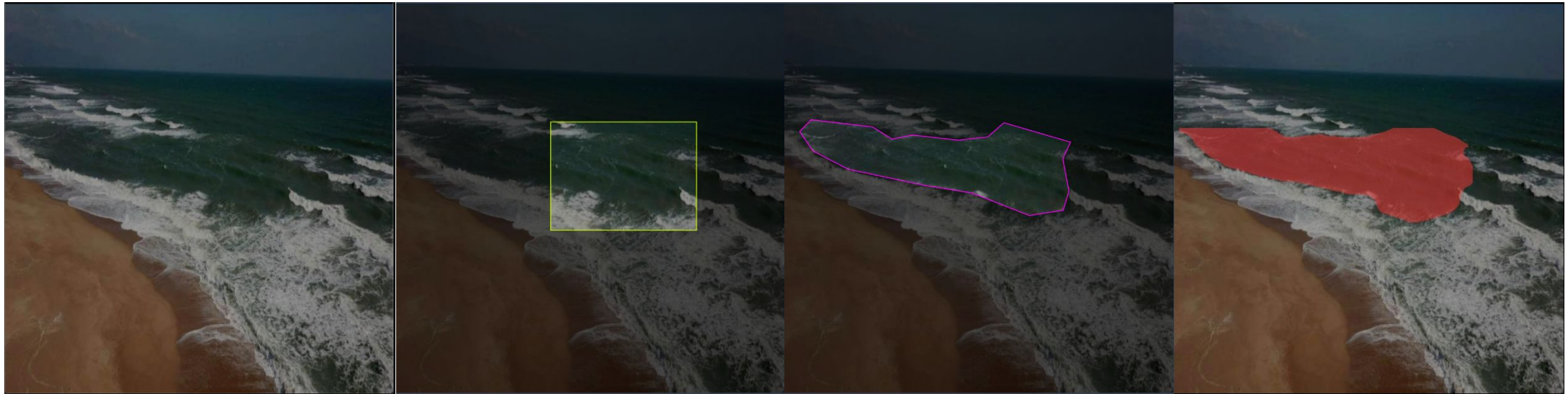
1. The original photo, 2. Existing bounding box annotation, 3. Our ground-truth annotation for instance segmentation, 4. Our prediction. This example highlights how bounding boxes may exclude relevant parts of the rip currents while also incorporating surrounding noise.
