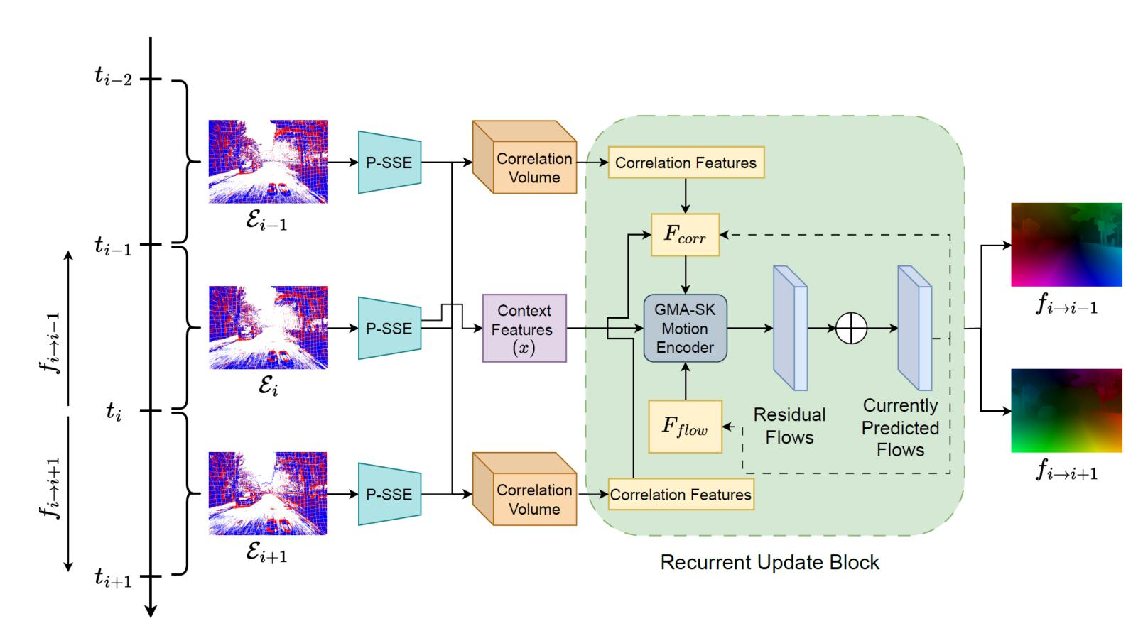
A simplified block diagram of the P-SSE encoder for tri-frame (E-TROF) case. Perturbed "A" matrix is used and the P-SSE is pretrained on ImageNet, then used in the following architecture
