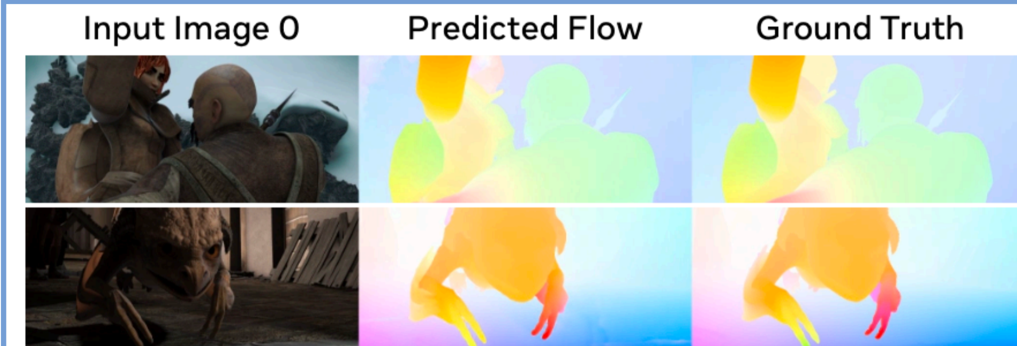
Optical flow on Sintel using the same tracking model. Predicted flows closely match ground truth even under large motion, occlusions, and clutter.
