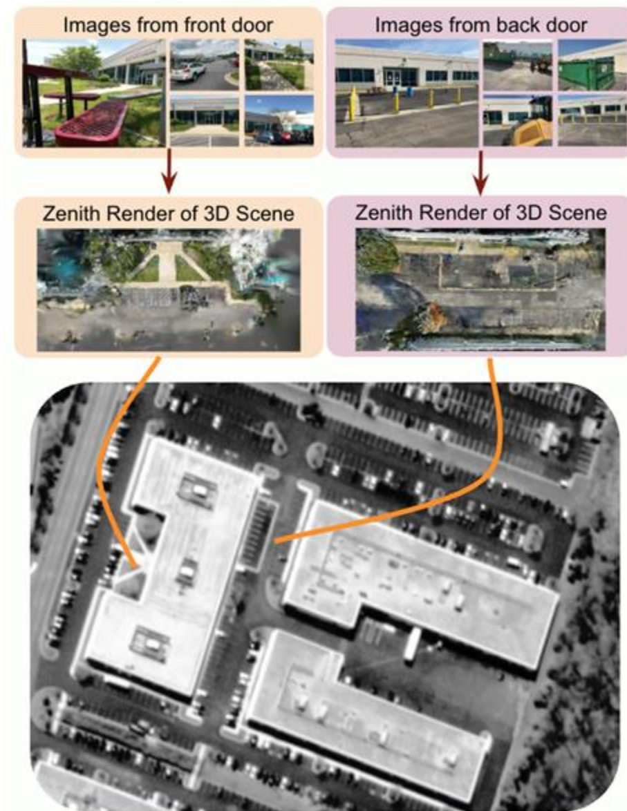
Ground-to-Satellite Alignment: Wrivinder reconstructs 3D geometry from ground images and aligns zenith renderings to satellite imagery.
