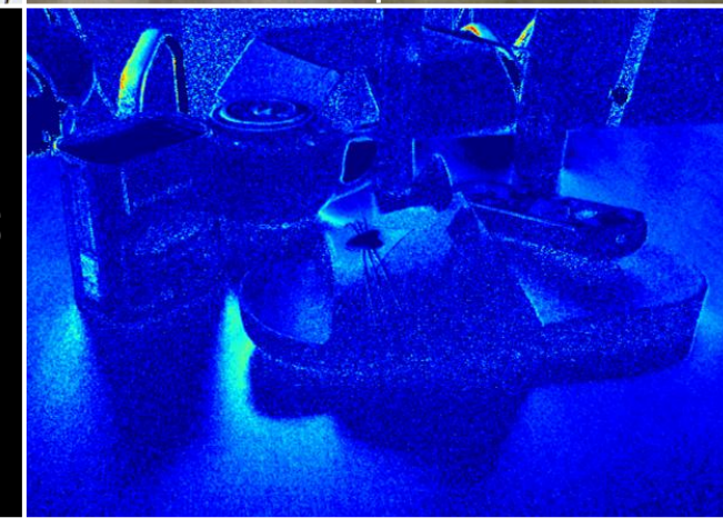
SPECULAR HIGHLIGHTS ARE LINEARLY POLARIZED
